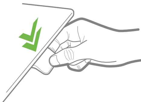
Figure 6 Double-tap the DPI to drive the desk to a pre-set favourite position
