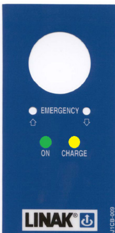
When connected to AC and charging battery
